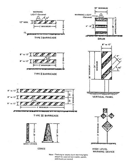
E. Barrel or Drum Application. Barrel or drums are an effective traffic control device, particularly for use in construction areas.
